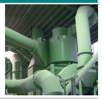
Gas centrifugal separators have a simple design, are robust, cost-effective and have low-maintenance operation.
